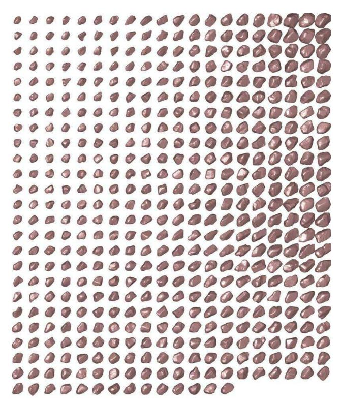
**Figure C.8**: Refined visual hulls of the data set consisting of 494 garnets used in a sieving experiment described in Chapter 10. Each visual hull is formed from 90 views of the stone obtained by merging 15 runs of 6-view silhouette sets. The 6-view silhouette sets were captured using the six-camera setup described in Chapter 5.
