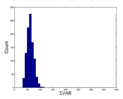
Figure 10.6: Histograms of  $\Sigma$ VAR values computed directly from sieve histograms with 1000 trials of random permutations of the 15 bin values for each stone. The  $\Sigma$ VAR value of 393.0 computed from the original data is indicated with a vertical line.
