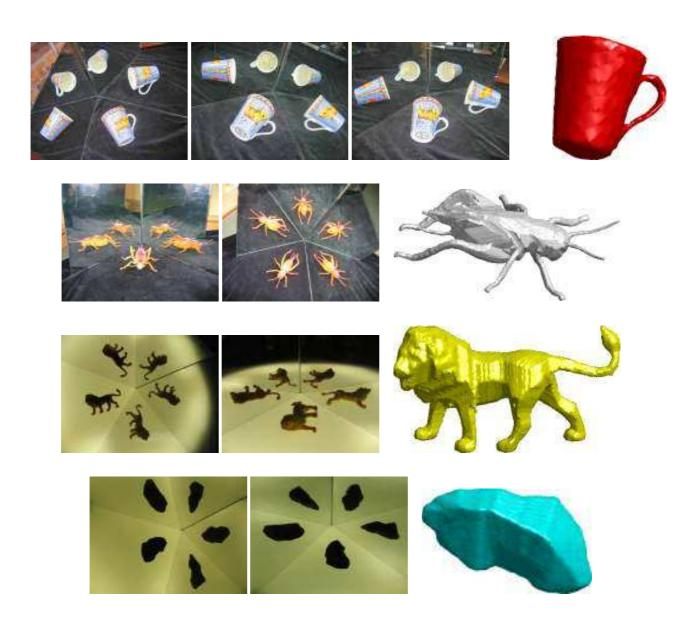
**Figure 4.10**: Visual hulls computed using the proposed two-mirror setup. Input images are shown in the to the left, and the resultant visual hulls are shown to the right. From top to bottom: a cup, a toy locust, a toy lion, and a piece of gravel. Black velvet was used as a background for the cup and the locust, whereas a backlight was used for the lion and the gravel.
