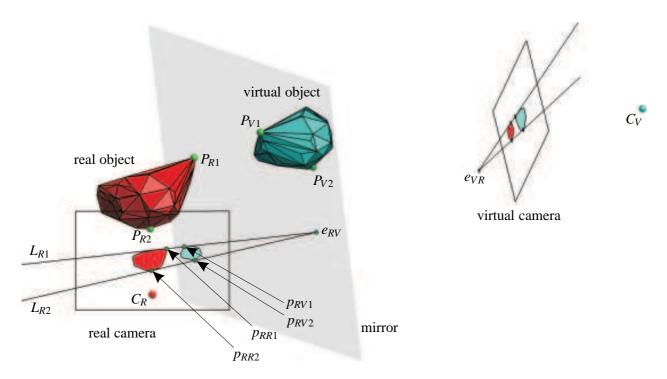
**Figure 4.3**: A camera viewing an object and its reflection. The epipole corresponding to the virtual camera can be computed from the silhouette bitangents  $L_{R1}$  and  $L_{R2}$ .
