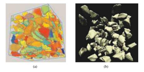
**Figure 2.2**: Computer simulations of concrete using 3D shapes based on real particles: (a) modelling concrete flow (picture from Bullard et al. [20]), (b) simulation of coarse aggregate in a mortar matrix flowing under mixing forces (picture from Garboczi et al. [52]).
