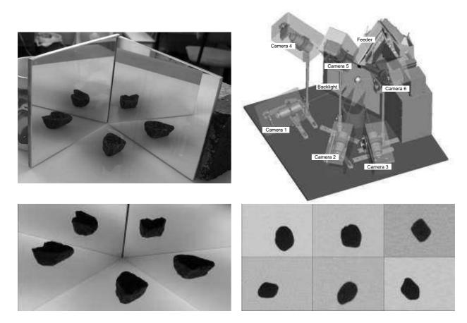
**Figure 1.1**: The two image capture setups considered in this thesis (*top*), and examples of corresponding captured images (*bottom*). The two-mirror setup (*left*) provides a simple low cost means of capturing silhouette sets of stones, whereas the six-camera setup (*right*) enables high throughput imaging.
