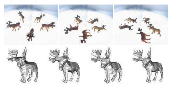
**Figure 6.11**: Reconstructing the 3D shape of a toy moose. The top row shows the three input images, and the bottom row shows the corresponding 5-view visual hulls. The rightmost visual hull is formed from the merged 15-view set.
