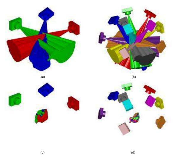
**Figure 3.2**: More accurate shape from additional views: (a) visual cones from three silhouette views, (b) visual cones from ten silhouette views, (c) the visual hull from the three silhouette views, (d) the visual hull from the ten silhouette views.
