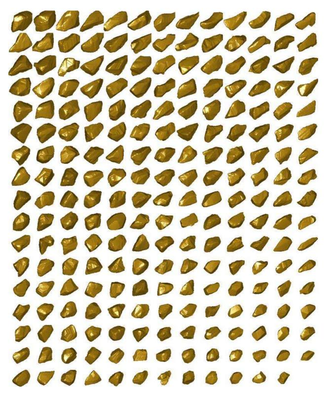
**Figure C.1**: Refined visual hulls of the data set consisting of 220 pieces of gravel. Each visual hull is formed from 15 views of the stone obtained by merging three runs of 5-view silhouette sets. The 5-view silhouette sets were captured using the mirror setup described in Chapter 4.
