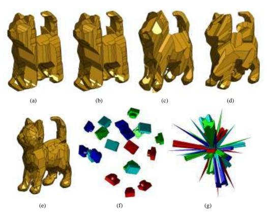
**Figure 6.10**: Visual hull models of a toy cat: (a)–(d) four models each built from five silhouettes, (e) the model built from the 20 silhouettes used in (a)–(d) after the poses of all silhouettes have been determined in a common reference frame. The camera poses corresponding to the twenty views are shown in (f), and the visual cones are shown in (g).
