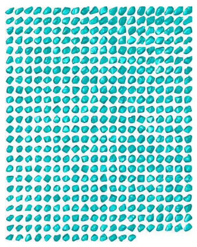
**Figure C.3**: Refined visual hulls of a portion of the data set consisting of 1426 naturally-occurring (uncut) gemstones. Each visual hull is formed from 60 views of the stone obtained by merging 10 runs of 6-view silhouette sets. The 6-view silhouette sets were captured using the six-camera setup described in Chapter 5. (The other stones from the data set are illustrated on pages 223 and 224.)
