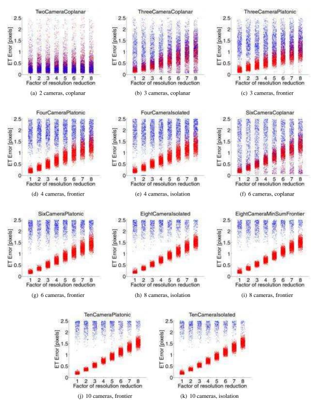
**Figure 7.16**: Plots of match values (red) and mismatch values (blue) for different camera configurations. Different levels of quantisation noise are shown, corresponding to different degrees of resolution reduction from the original image resolution. Cameras are configured to fulfil the frontier point criterion (frontier), the direction isolation criterion (isolation), or to have coplanar optical axes with even angular distribution about 180° (coplanar).
