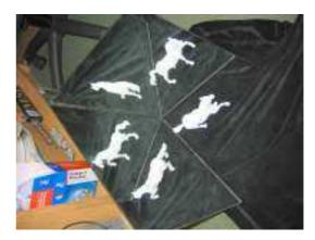
**Figure 4.2**: Two images of a two-mirror setup positioned so that five views of the object can be seen. Note that the camera has moved between shots, but the mirrors and object have not moved.
