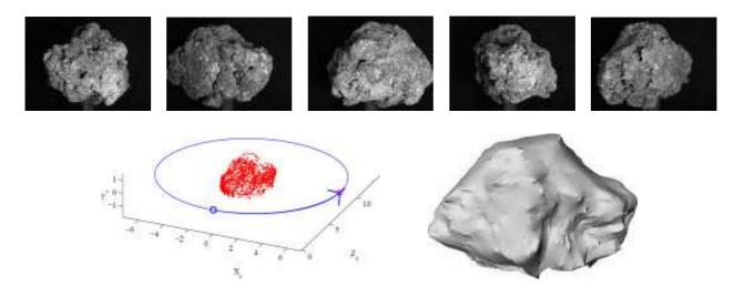
**Figure 2.8**: Rock shape reconstruction. Images are captured as a rock is rotated on a turntable. The top row of images shows 5 of the 226 images used. The camera trajectory and reconstructed 3D points (*bottom*, *left*) and triangular mesh model formed with Delaunay triangulation (*bottom*, *right*) are also shown (pictures from Bouguet [13]).
