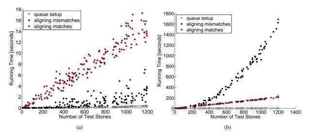
**Figure 9.2**: Running time for batch matching different numbers of stones: (a) using the VEMH and moments up to order 3, (b) using the CDRH and moments up to order 1. The running time consists of time spent setting up the priority queue and applying pose optimisation to matches and to mismatches.
