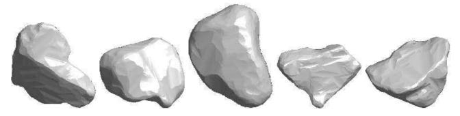
**Figure 10.3**: Refined visual hull models of stones whose minimum sieve bin is smaller than the minimum cylinder diameter by the largest amount.
