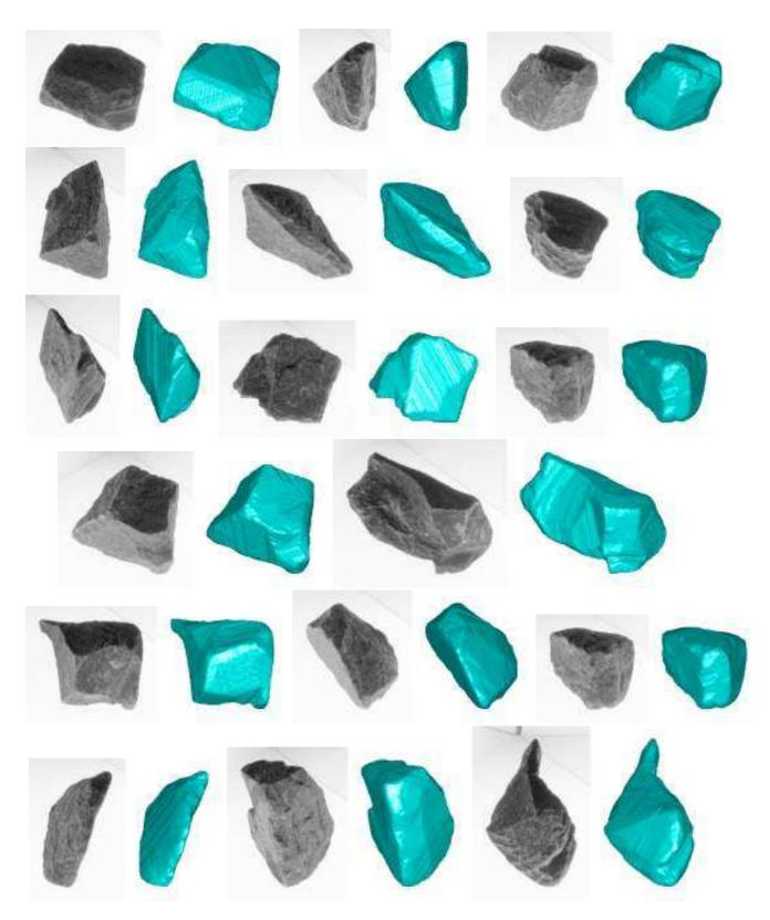
Figure 6.14: Images of pieces of gravel with visual hulls shown from the same viewpoint. The visual hulls were formed from three images of the stones, yielding  $3 \times 5 = 15$  silhouettes for each visual hull.
