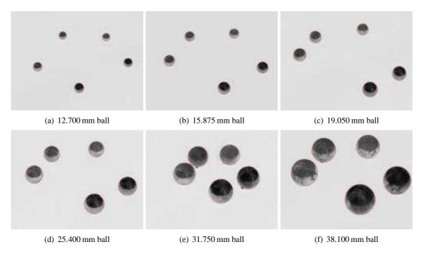
Figure 4.14: Six images of six ball bearings used for enforcing scale.
