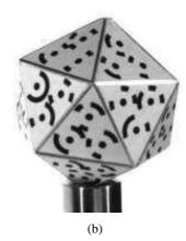
**Figure 5.7**: Two examples of calibration objects with coded targets: (a) a cube with 54 targets and 9-bit code bands, (b) an icosahedron with 60 targets and 10-bit code bands.
