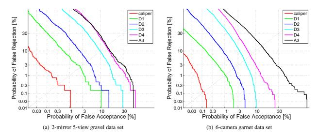
**Figure 8.8**: ROC curves derived from (a) the 2-mirror 5-view gravel data set, and (b) the 6-camera garnet data set for caliper signatures and for the shape functions proposed by Osada et al. [104]. One million samples of each shape function of Osada et al. was used for each VEMH. This value was found to be sufficiently large so that further increases showed negligible improvement in accuracy.
