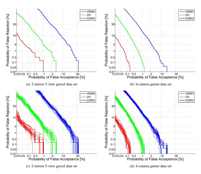
**Figure 8.7**: ROC curves derived from (a) the 2-mirror 5-view gravel data set, and (b) the 6-camera garnet data set for caliper signatures computed using different means to approximate the 3D convex hulls of stones: VEMHs, visual hulls, and CDRHs; (c) twenty bootstrap curves drawn from the data presented in (a); (d) twenty bootstrap curves drawn from the data presented in (b).
