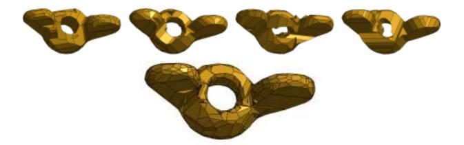
**Figure 6.9**: Visual hulls of a wing nut. The top row shows four 5-view visual hulls. The bottommost illustration shows the refined 20-view visual hull obtained by merging the four 5-view silhouette set into a single large set containing 20 silhouettes.
