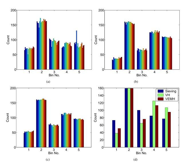
**Figure 10.1**: Histograms for (a) sieving, (b) minimum cylinder of the visual hull, (c) minimum cylinder of the VEMH, and (d) mean bin counts for 15 runs of the three sizing methods. Each run is represented by a different colour bar for histograms (a)–(c).
