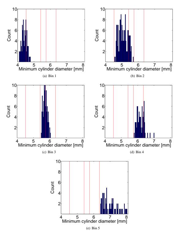
**Figure 10.2**: Histograms of minimum enclosing cylinder diameters for 90-view visual hulls of garnets whose minimum sieve bin is (a) Bin 1, (b) Bin 2, (c) Bin 3, (d) Bin 4, (e) Bin 5. Vertical lines indicate the sieve aperture diameters.
