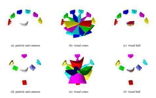
Figure 5.2: Six cameras observing a banana-shaped particle: (a)–(c) show cameras with coplanar optical axes, (d)–(f) show cameras based on a Platonic solid geometry. Note that the coplanar cameras yield a visual hull model that is much larger than the particle: the extra volume is due to the saddle-shaped region of the particle. The cameras based on a Platonic solid geometry yield a visual hull model that is a relatively close approximation to the particle.
