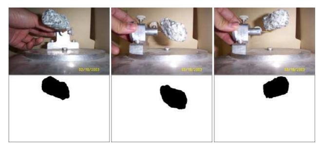
**Figure 2.3**: Three images from a sequence captured using a turntable device for rotating individual rocks about two different axes (*top row*), and the corresponding manually segmented silhouettes (*bottom row*) (pictures from Lau [72]). The images were used to investigate volume prediction from multiple silhouette views.
