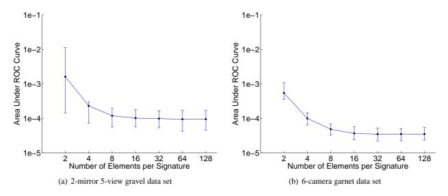
**Figure 8.4**: Plot of number of signature elements versus area under the ROC curve for (a) the 2-mirror 5-view gravel data set, and (b) the 6-camera garnet data set. Error bars represent 95% confidence intervals computed using the subsets bootstrap. Six icosahedron subdivisions were used to compute 3646 directions for caliper diameter samples from each VEMH. Note that nonlinear axes have been used.
