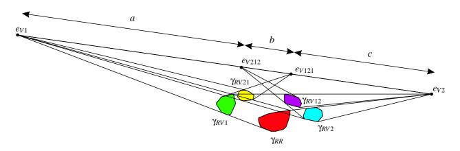
**Figure 4.5**: Computing epipoles  $e_{V1}$ ,  $e_{V2}$ ,  $e_{V121}$ , and  $e_{V212}$  from the silhouette outlines in an image.
