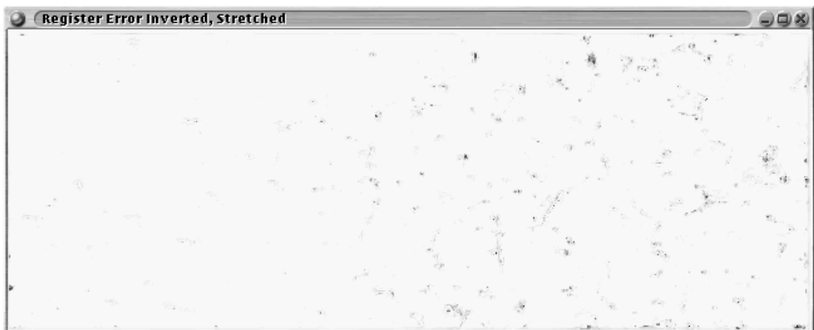
(c) Registered error, stretched. Energy in error image is 4 054 200.
