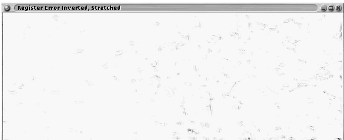
(c) Registered error, stretched. Energy in error image is 2 208 070
