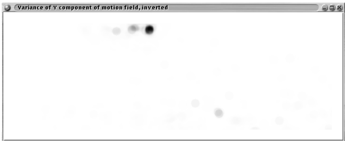
(b) Variance of the Y component of the motion field, inverted.
