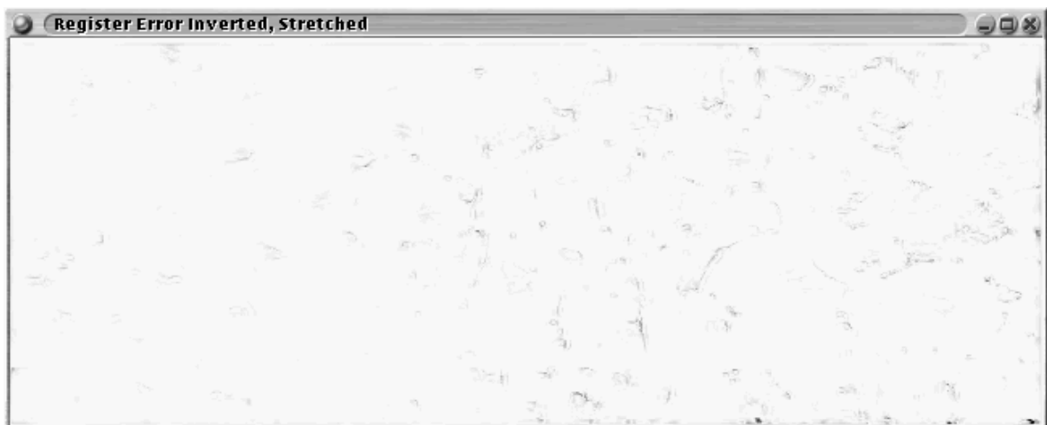
(c) Registered error, stretched. Energy in error image is 1 774 367.
