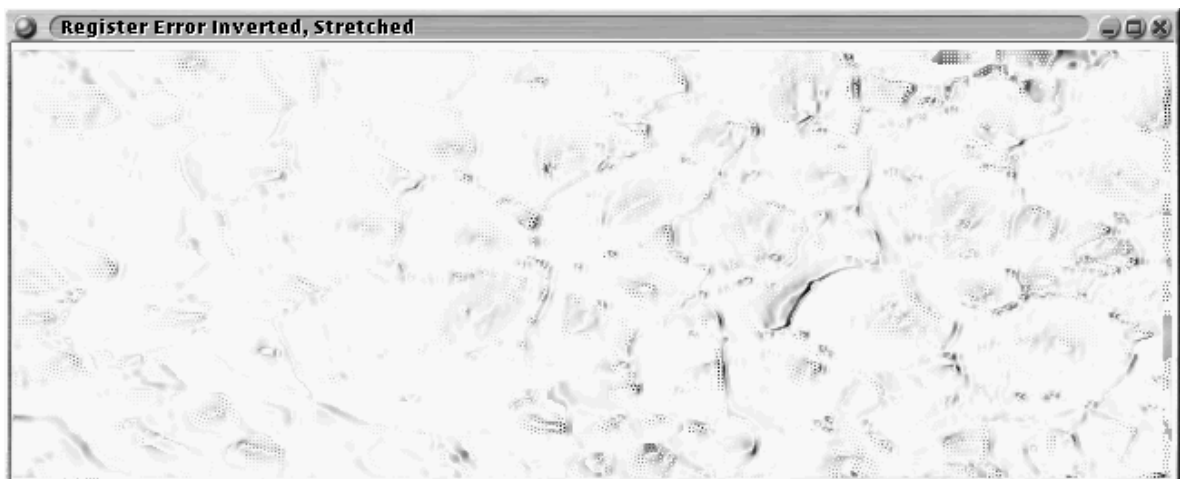
(c) Registered error, stretched. Energy in error image is 27 572 317.
