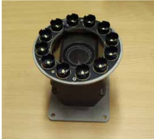
Figure 3.6: SmartFroth camera in waterproof housing with ring of LEDs for consistent illumination.
