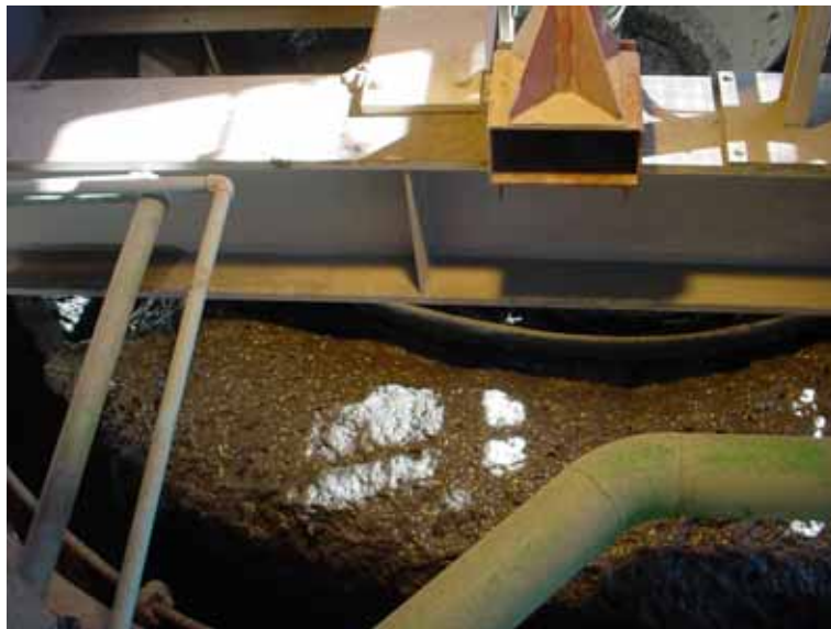
Figure 3.4: Patches of sunlight falling onto the field of view of the camera system results in poor measurements and should be avoided.
