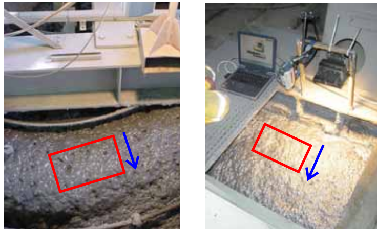
Figure 3.9: Fields of view for two cameras. The red rectangles mark the fields of view and the blue arrows the direction of froth flow.
