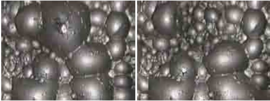
Figure 3.17: Two consecutive frames of video footage. Note the bubble that has burst.
