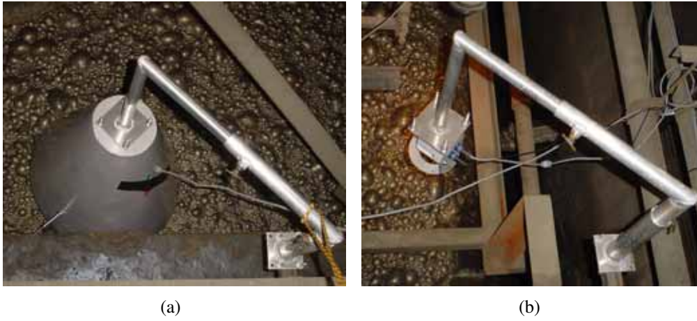
Figure 3.7: A long-term installation of the SmartFroth camera system. (a) camera, lighting and hood. (b) camera and lighting only.
