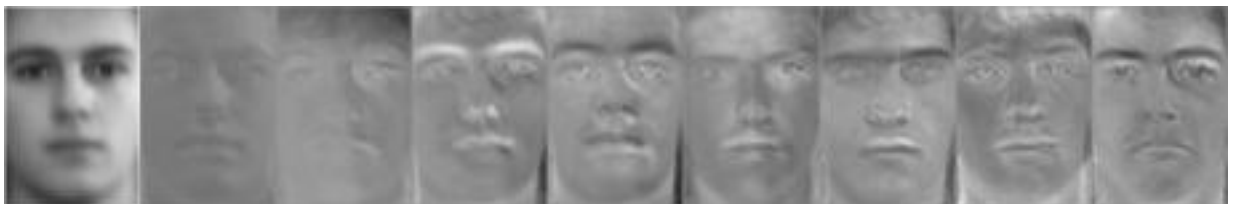
Figure 5.10: The average face and the first 8 eigenfaces generated from applying principal component analysis on the training set of 46 face images.
