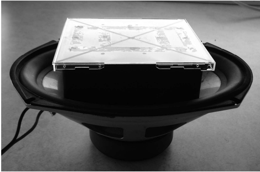
Figure 9.1: The vibration platform used for testing accelerometers.
