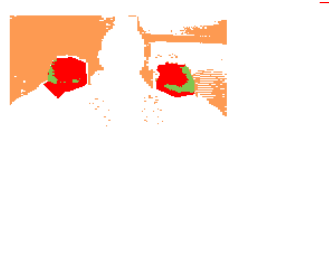
Figure 4.7. Incorrect classifications using the explicit skin-colour segmentation.
