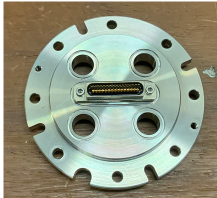
(c) The bottom flange with the DC connector attached.
