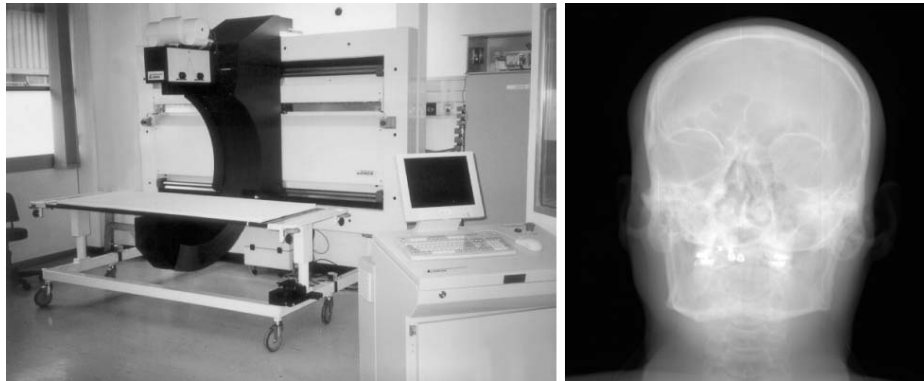
Figure 6.1: LODOX digital X-ray machine and example of an X-ray image
