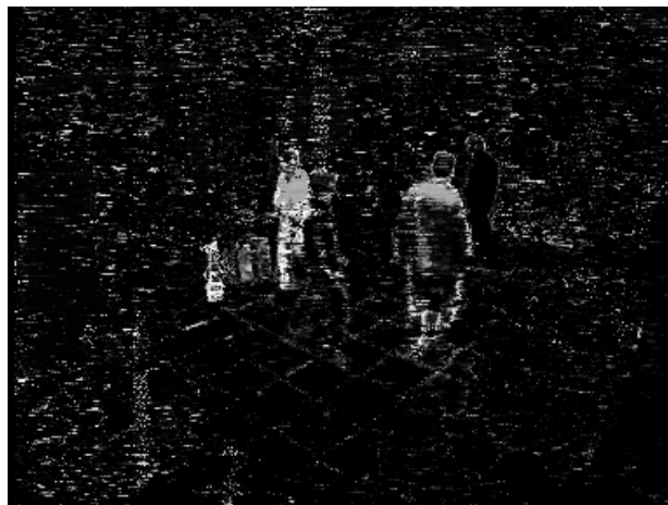
Figure 5.2: The basic pixel classification map for the first person as generated by Gaussian Mixture Models trained in L^*a^*b space.
