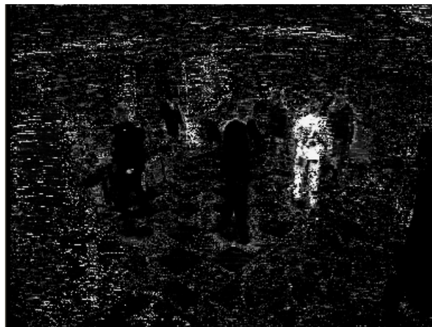
Figure 4.11: Pixel classification of the white person using GMMs trained with RGB data.
