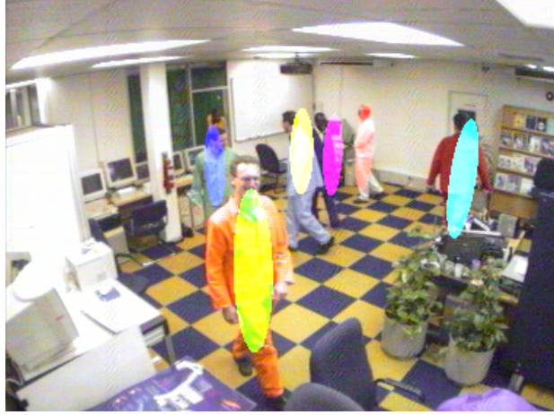
Figure 4.4: The image projection of such a hypothesis will be compared to the data image. If the hypothesis is good, then the target objects which the ellipsoids represent will occupy the same region in image space as the people.
