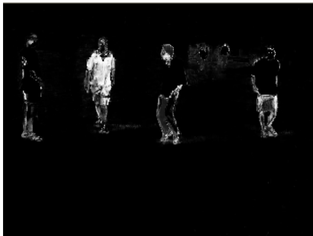
Figure 4.20: Pixel classification of the fourth person using GMMs trained with L^*a^*b^* data.
