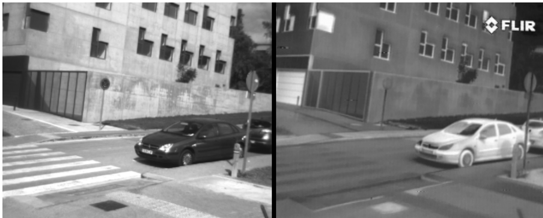
Figure 2.3: CVC Multimodal Stereo Dataset (2). The hand-rectified images are taken from two rigidly mounted cameras. The Sony Charge-coupled device (CCD) camera and the PathFindIR FLIR camera produce 640 \times 480 and 534 \times 426 pixel images respectively. Once the images have been rectified they are both 506 \times 408 [34, 35].
