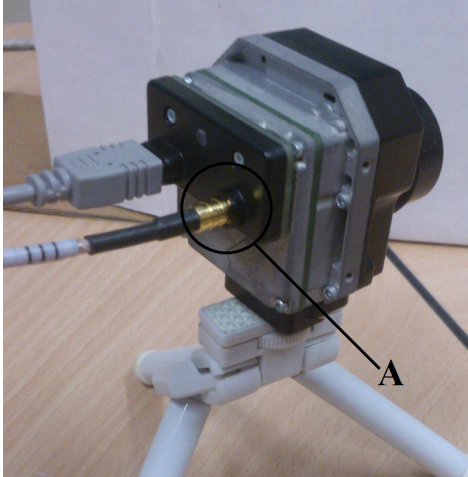
(a) The Tau module. A shows the analogue video output micro coaxia cable; the mini-USB port powers the device.
